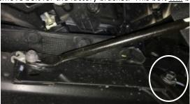
3) Identify the correct bracket for the side of the vehicle currently being worked on. Cube lights can be mounted onto the bracket at this point.
