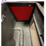
Peel adhesive backing and place bracket into saddle bag.
