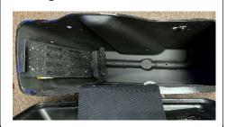
4. Once amplifier has been installed, place cover on bracket using supplied push pins.
