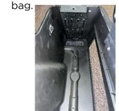
4. Once amplifier has been installed, place cover on bracket using supplied push pins.
