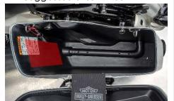
2. Peel adhesive backing and place bracket into saddle bag.
