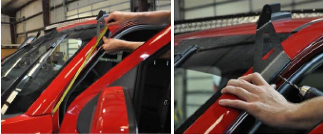
4. Use the supplied 3/16" rivets to secure the light brackets. **NOTE: Repeat steps on the driver side.**
