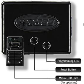
† AXSWC Unit/Box with the reset button between the LED and Micro USB Port.
