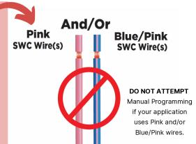
If the automatic programming sequence fails even after following the **Troubleshooting** steps above, the AXSWC interface **may be** manually programmed to the vehicle under certain conditions.
